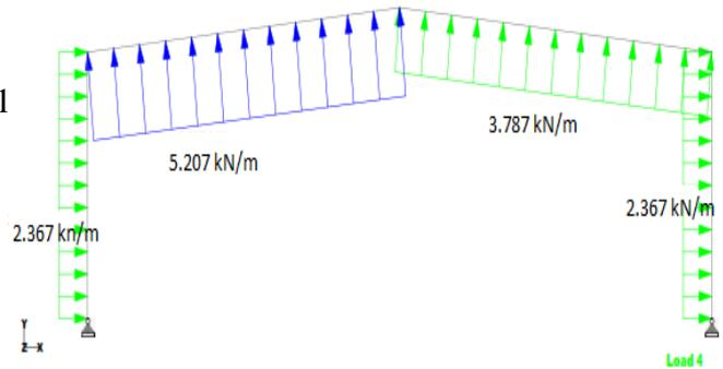
Fig 3.2: Wind load @0° for(C<sub>pi</sub> =+0.2) Left side wind ward
