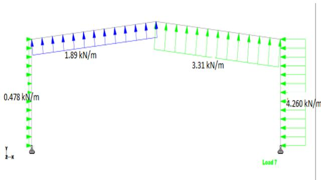
Fig 3.5 : Wind load @0° for(Cpi =-0.2) Right side wind ward
