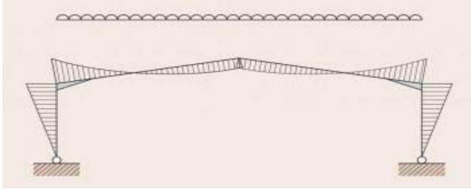
Fig. . 1.1 Bending moment diagram for hinged support
