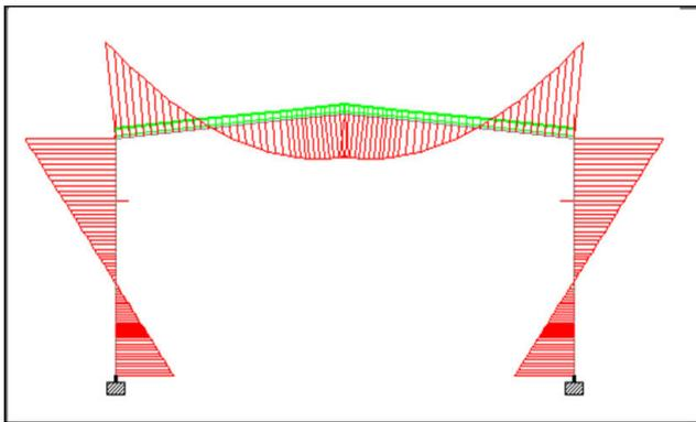
Fig.1.2 Bending moment diagram for fixed support
