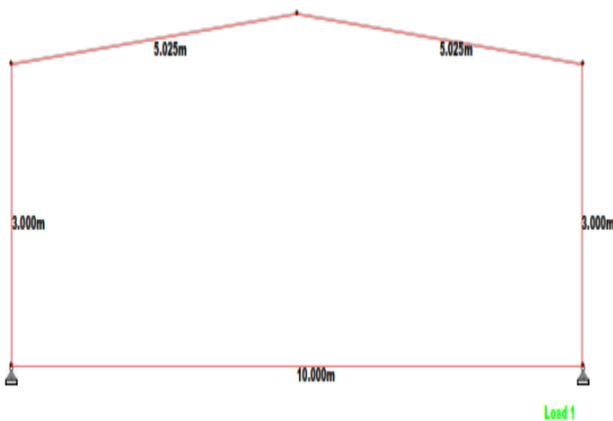
Fig.3.1 Elevation of 10 m span frame
