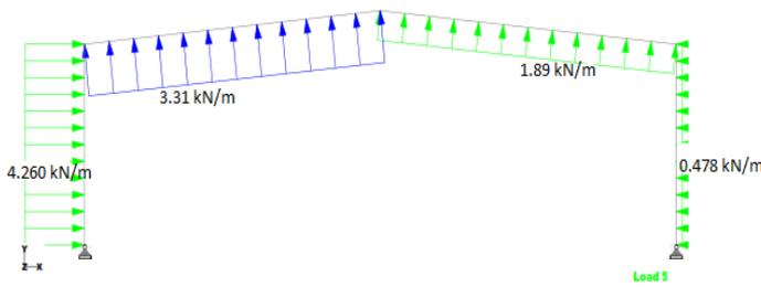
Fig 3.4 : Wind load @0° for(Cpi =-0.2) left side wind ward
