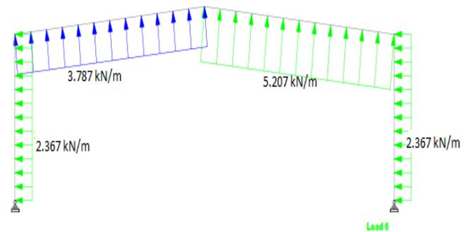
Fig 3.3 : Wind load @0° for(C<sub>pi</sub> =+0.2) right side wind ward
